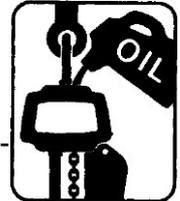
To avoid oil leak, make sure to firmly fasten drain plug.
